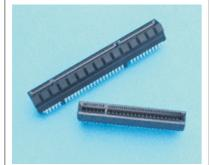
The card-edge connectors utilize an "eye-of-needle"-compliant section for termination to a backplane. The pressfit connectors are targeted for use on 2.36mm (0.093") to 4.19mm (0.165") thick PCBs. By using press-fit connectors, manufacturers can avoid soldering problems and improve manufacturing yields when implementing I/O slots on thick backplanes. RoHS-compliant connector versions are available.
